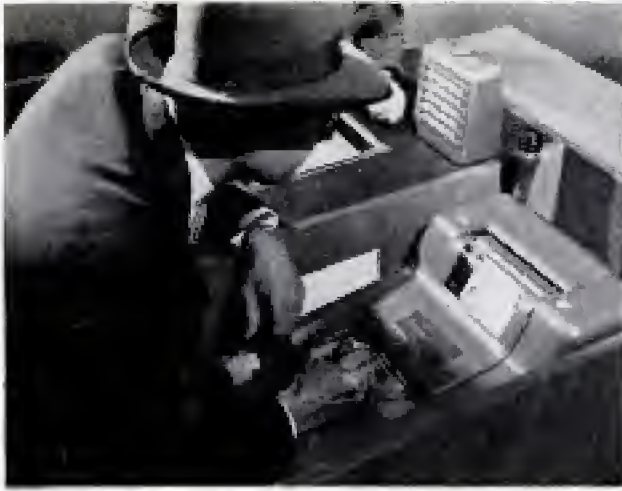
Depositor signs withdrawal slip on telautograph. Signature is duplicated by similar unit at main bank
